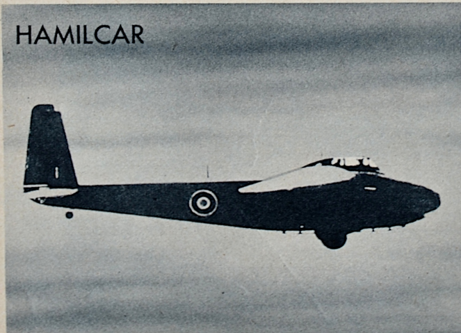
HEAVY BODY , huge wing, distinctive high fin and rudder serve to distinguish the Hamilcar. Undercarriage resembles that of U. S. glider types.
