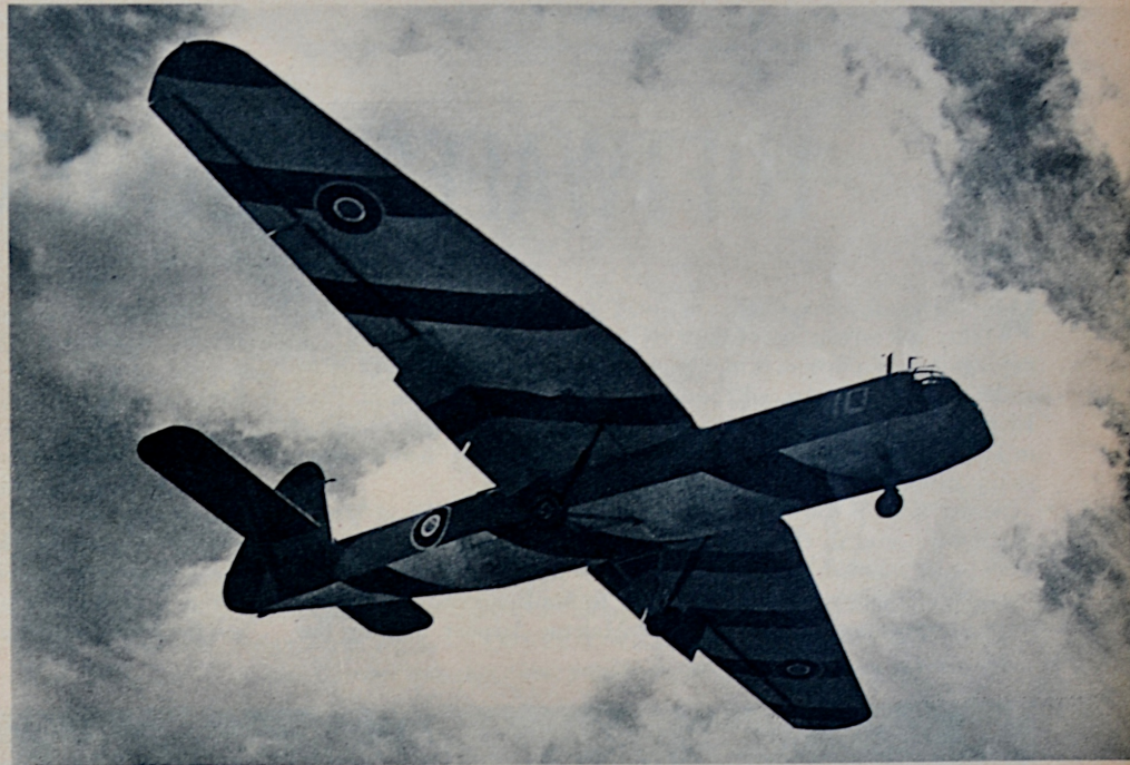
FIRST GLIDER to have tricycle landing gear, Horsa may also be seen without an undercarriage. Horsas were used along with CG-4A's in airborne phase of attack on Sicily for their first operational test.
